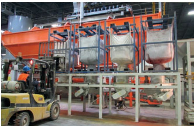
Figure 2 -- Above, an operator loads the ACT/Würschum TFW 90 dry-powder color metering system with a 2,000 lb super sack of pigment. With four basic colors, StoneBilt can reproduce any natural earth tone for its wet cast retaining wall and paver hardscape products. The color metering system is integrated with the ACT PCS programmable controls, providing high accuracy and consistency in color and recipe reproduction. Dry pigment is "slurrified" and pneumatically conveyed to the appropriate mixer. Moisture content is continuously monitored and automatically adjusted by the ACT Hydromat microwave probe in each mixer.
